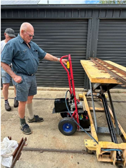
Hydraulic traverser, 5" and 7 ¼" catered for. Overall length of the traverser is approximately 2400mm.
