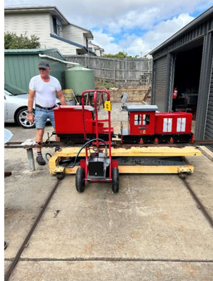
Hydraulic traverser track connection may require a joiner piece from your vehicle to the traverser track. The club/members have some joiners available that may suit your vehicle.
