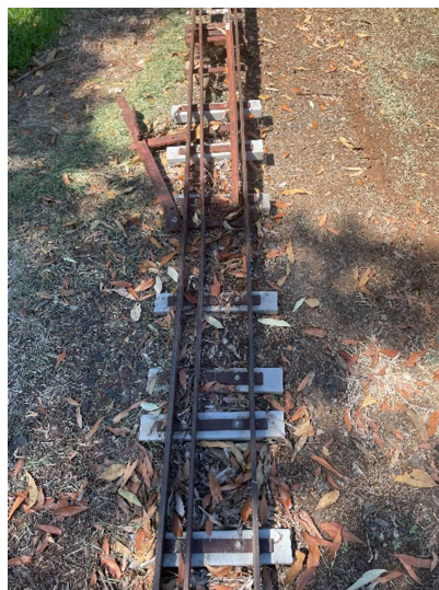
The 5" to 7 ¼" transfer point. Drivers check position of the points before proceeding.
